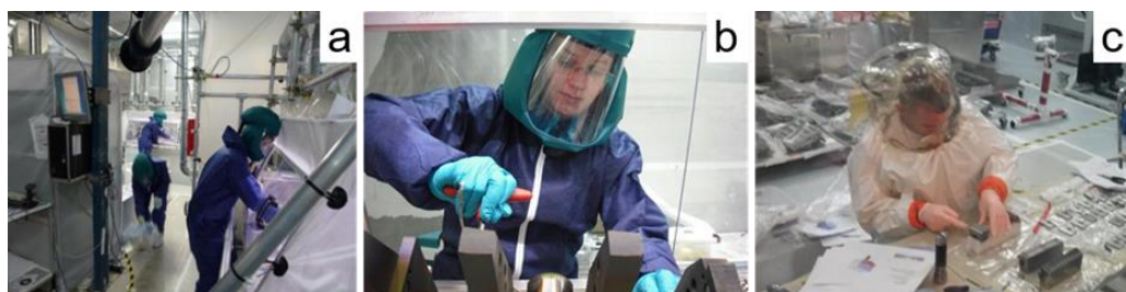
Figure 6. Operatives working in the Beryllium Handling Facility [81], a facility for supporting JET operation and maintenance. (a) and (b) Operative are wearing air inflated hoods equipped with a filter, disposable coveralls, rubber boots with overshoes and several pairs of gloves including a sacrificial top layer which is changed periodically. Work on JET components is carried out in ventilated slit boxes to minimise the spread of contamination and exposure to operatives. (c) Where it is not possible to work within a slit box, operatives wear a full containment suit with dedicated pressurised air supply.
