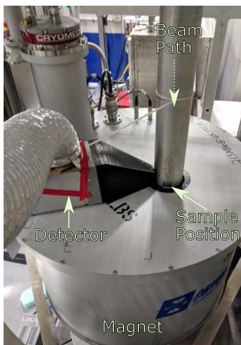
Figure 4: Apparatus in the data taking position. Detector shown with a 3-D printed shield to reduce background.
