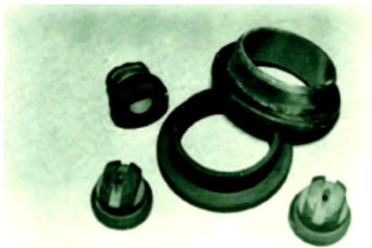
Fig. 10. Ceramic articles made of black ceramics, obtained by direct SHS-sintering.
