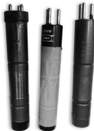
FIG. 1. Sample Geiger Muller tubes salvaged from legacy Victoreen CDV 700 survey instruments recovered from fallout shelters.
