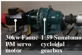
Fig. 3. Fanuc PM servo motor connected in series with a 59:1 Sumitomo cycloidal gearbox (CHHJ-4225Y-59-320TC). [27]
