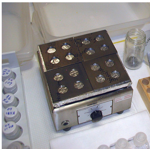
Fig. 6 Hot plate used for plating alpha samples and columns used for separation
