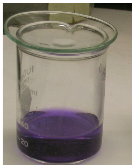
Fig. 12 Solution of Pu(III) in HCl media after metal dissolution
