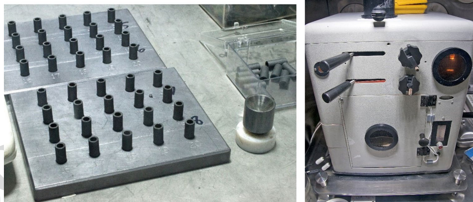
Fig. 8 Graphite cup electrodes used for sample analysis and an Arc chamber used for striking an arc in sample analysis
