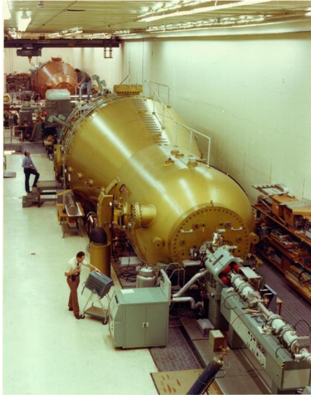
Figure 4 – View of the two BNL Tandem accelerators. Each of them can deliver ion beams either of the two target rooms.
