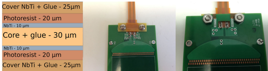
Fig. 2 Left: Cross-sectional diagram of the layers of the NbTi stripline. Center: Top of the LC board PCB connected to the stripline with ultrasonic solder joints. Right: Bottom of the LC board PCB connected to the stripline with ultrasonic solder joints (Color figure online)
