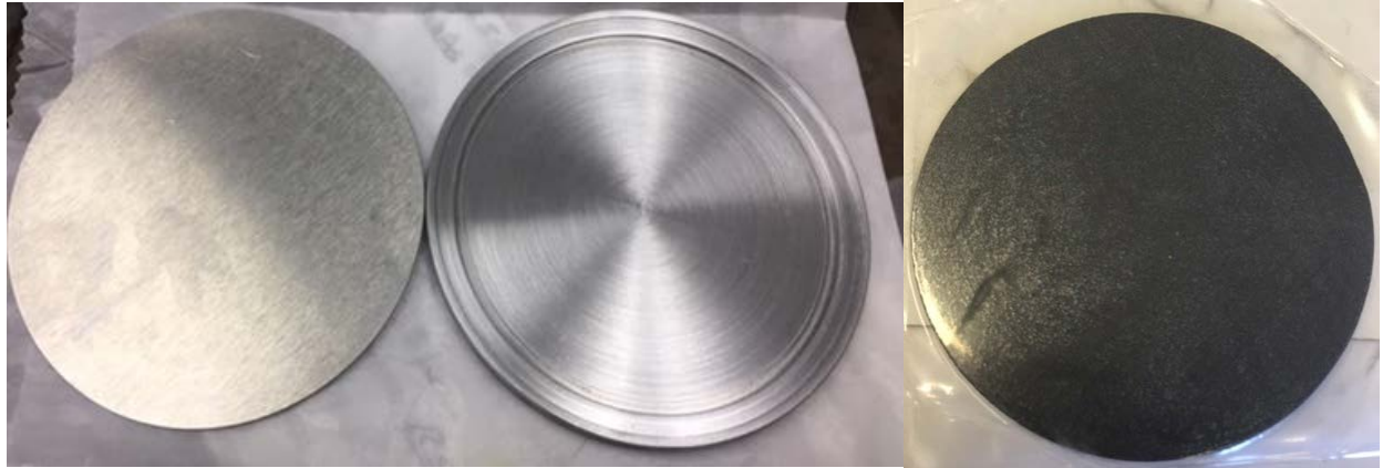
Figure 3. Production target components (from left to right): aluminum window, aluminum can body with machined counter-bore, and arsenic metal sputtering target (d x h = 2.375" x 0.032"; 60.325 mm x 0.8128 mm).
