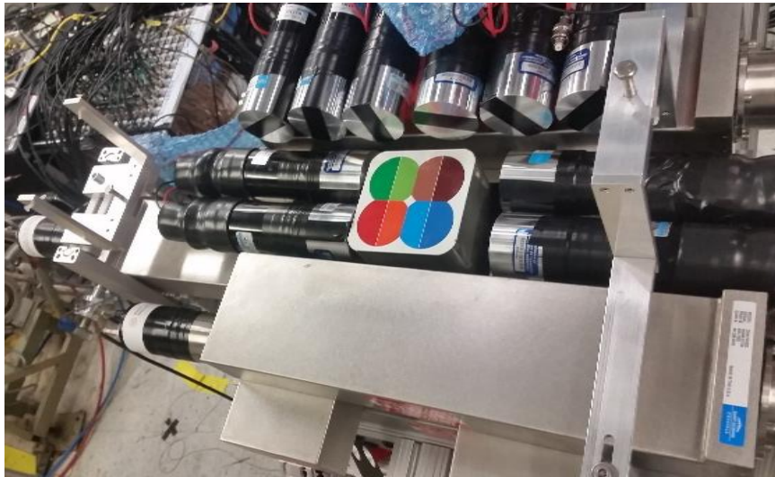
Fig. 1. Picture of a portion of the \gamma -ray detection used with VANDLE at the OLTF. The beamline placed within the square brackets has been removed; beam enters from left to right. The large rectangular detectors are NaI(Tl), the central square shaped detector with circular stickers is the HPGe from CLARION, and the cylindrical detectors are HAGrID. Some detectors on beam right (bottom side of image) have been removed. VANDLE is not visible as it is placed above the \gamma -detection array.
