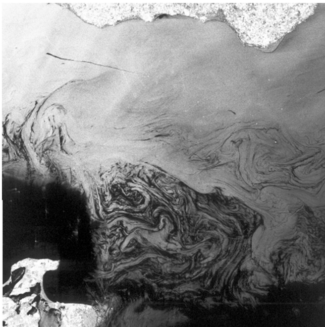
Fig. 9. SAR image acquired by ERS-1 satellite on 16 April 1994 at 21:04 UTC over the Baltic Sea (Pommerian Bight). Visible is in the lower left hand section the German island of Ruegen and on the top the Swedish coast. This SAR image shows biogenic slicks entrained by a complex surface current field. The dark area to the left is very likely an area completely covered by biogenic slicks. Note also in the upper left hand section the dark line with a bright spot at the end where the line is narrowest (to the right). It clearly results from oil spilled from a ship. Imaged area: 100 km \times 100 km.
