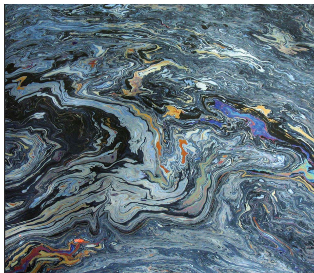
Fig. 2. Photo of a thin mineral oil film showing iridescent (rainbow) and silver sheens indicating different thickness of the oil film. (For interpretation of the references to color in this figure legend, the reader is referred to the web version of this article.)
