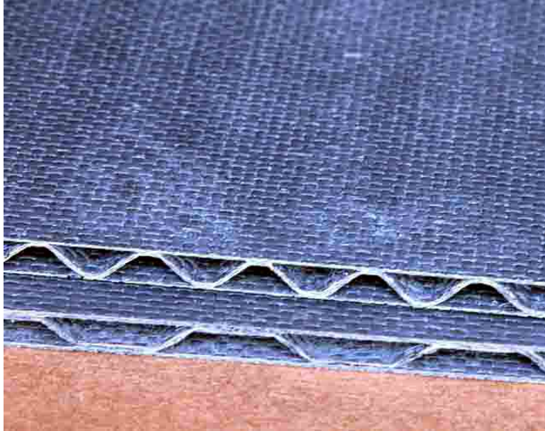
Fig. 3. Example of fluted core FCI structures made of continuous SiC fiber–reinforced SiC–matrix composites. (Courtesy: Rolls-Royce High Temperature Composites Inc.)
