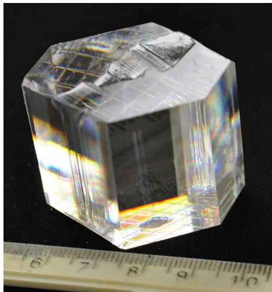
Figure 4. The final stilbene-d 12 crystal grown in the shape of a hexagon. The initial seed is still seen through the optically transparent material that does not show any visible defects. The crystal mass is 38 g with a height of 35 mm.
