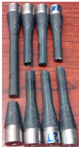
Figure 16: Specimens with failure in transition section (leftmost specimen) and mid-gage section.
