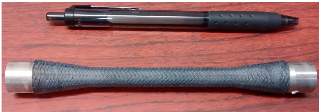
Figure 2: An axial tensile test specimen with steel end plugs.
