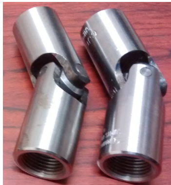
Figure 6: Swivel joints employed to minimize the bending which occurs due to irregular geometry of the specimen.
