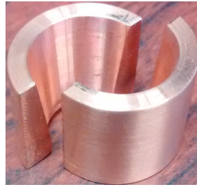
Figure 5: Annealed copper collets with tapered inner surface
