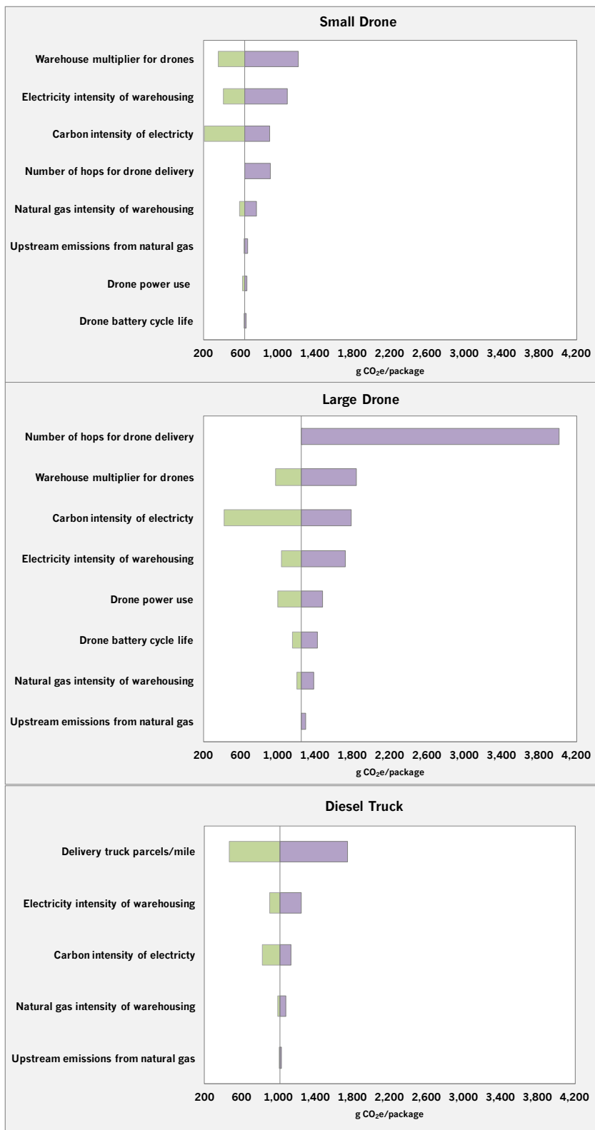
Figure 6: Sensitivity analysis: GHG emissions per packaged delivered for the quadcopter, octocopter, and diesel truck under the parameters listed in Table 2. Vertical lines mark the base case result for each mode. Green bars (stretching to the left of the line) show the decrease in emissions and purple bars (stretching to the right) show the increase in emissions given parameters Table 2.
