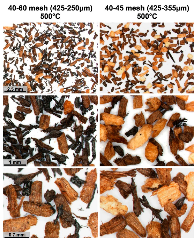
Figure 1. Reflected light stereoscope micrographs of unsorted pine chars. Two different size ranges, 40–60 mesh and 40–45 mesh, of milled loblolly pine particles were subjected to fast pyrolysis at 500 °C. The char particles display color and morphological heterogeneity suggesting they were subjected to pyrolysis under variable process conditions.
