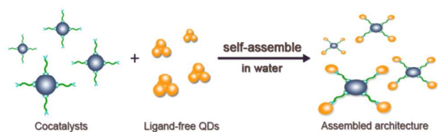
Scheme 1. Schematic illustration of the process of the self-assembled architecture between ligand-free QDs and Pt-nanoparticles in aqueous solution formed in situ .
