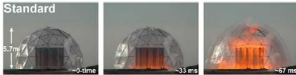
Figure 8: High-speed optical video images of hydrogen combustion for a 30% hydrogen/air mixture, ignited with a 40 J spark. Figure reproduced from Reference 48.
