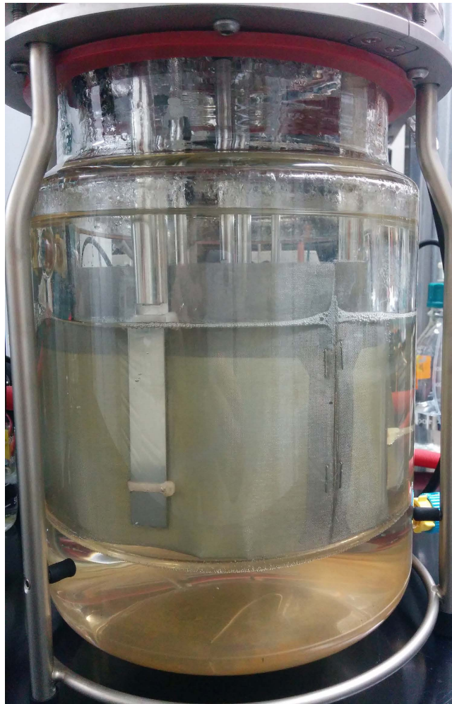
Figure 5. Bioreactor with stainless steel meshes adapted to baffles that support cellulose and biofilms, and were used for quick collection of sessile cells for RNA-Seq analysis.
