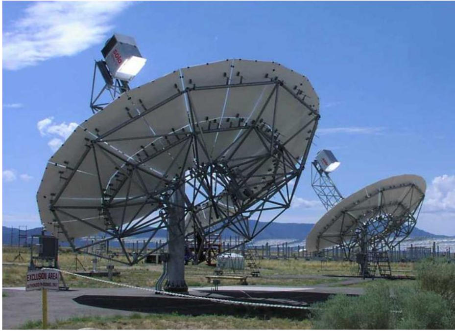
Figure 22. ADDS dishes with Mod 1 (left) and Mod 2 (right) at Sandia.[95] The Mod-2 system pictured is an off-grid water pumping unit.
