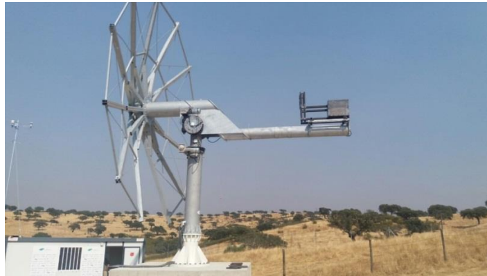
Figure 37. The steel structure for the BioStirling dish, without mirrors installed [136].
