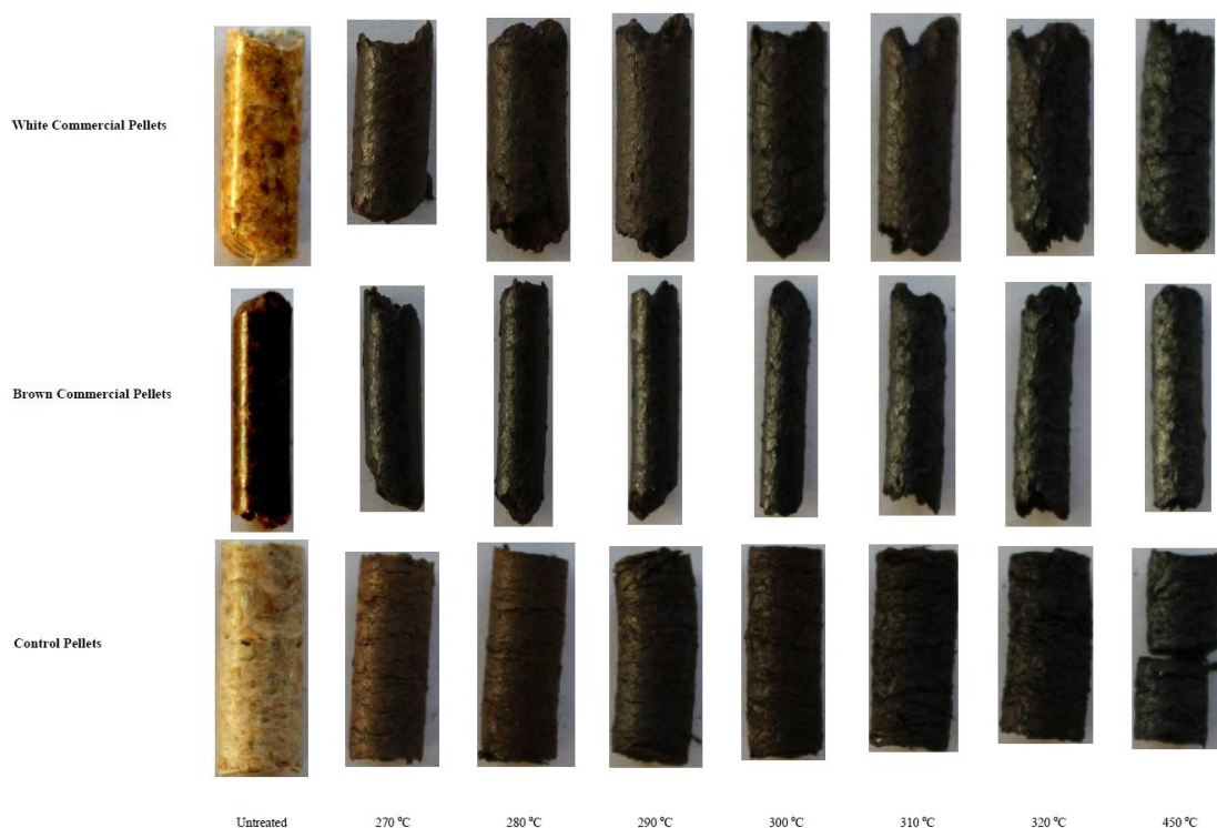
Fig. 1. Photo of torrefied wood pellets made from the torrefaction of wood pellets at different temperatures for 30 min.
