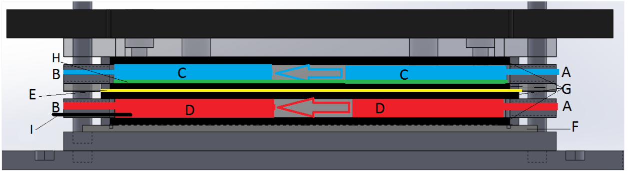
Figure 1. Schematic of the parallel electrochemical treatment system showing inlet (A) and outlet (B) ports for catholyte (C) and anolyte (D), Nafion membrane (E), working electrode (F), electrochemically inert gasket material (G), planar counter electrode (H), and reference electrode (I).
