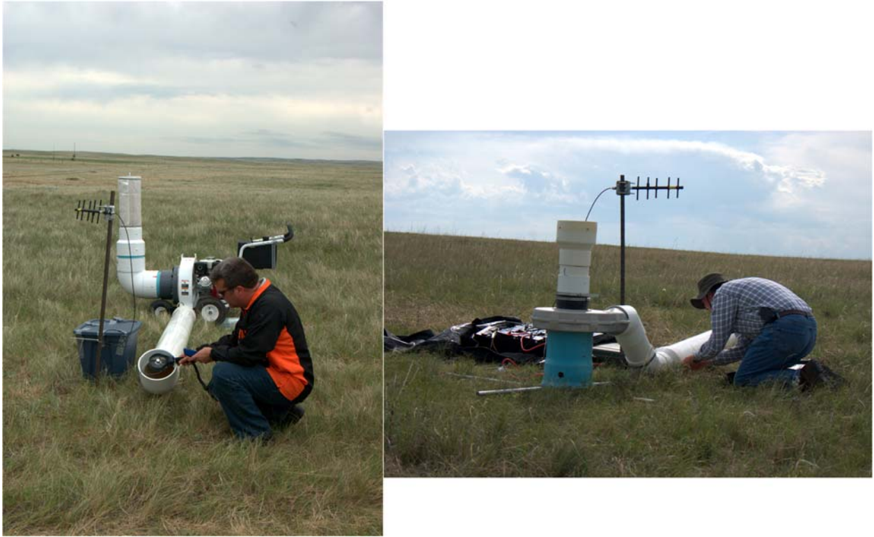
Figure 1: The image on the left shows the gasoline powered air sampler adapted from a leaf blower. The image on the right shows the air sampler adapted from a blower which is actuated by a DC electric motor. Note that in these images, the frame for the air filter is installed on the gasoline powered air sampler, but has not yet been placed on the electric air sampler.
