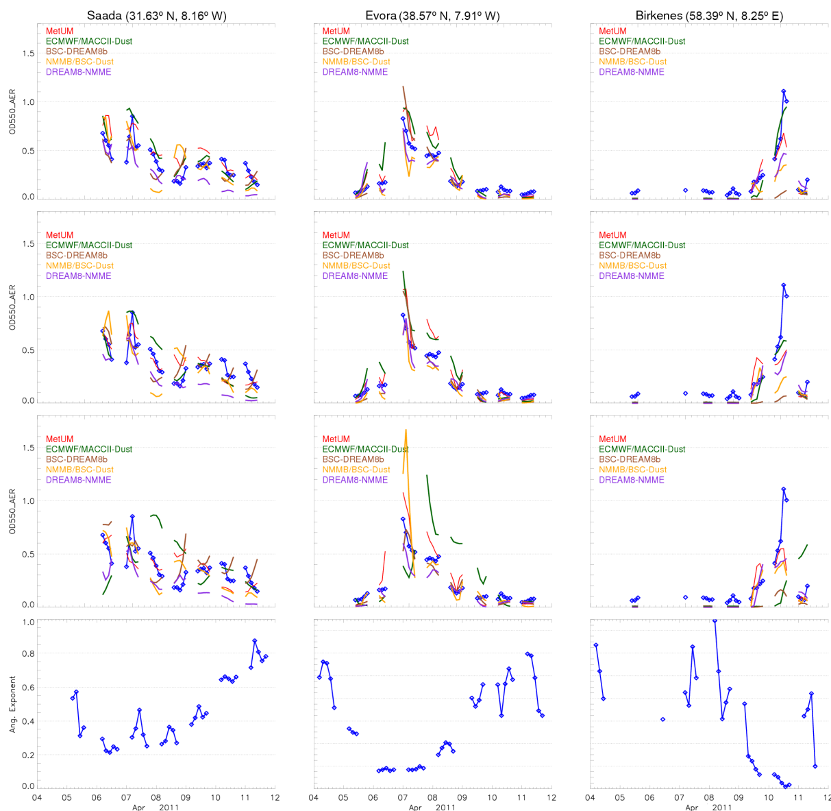
Figure 2. Total AOD at 550 nm at three selected sites from the AERONET network (blue line) and 24 (first row), 48 (second row) and 72 h (third row) forecasts of the models MetUM (red), ECMWF/MACC (green), BSC-DREAM8b (brown), NMMB/BSC-Dust (orange) and DREAM8-NMME (purple) are illustrated. The Angström exponent (dark blue dots) from the AERONET network at the three selected sites is included in the fourth row. Angström exponents < 0.75 indicate the dominance of desert dust.
