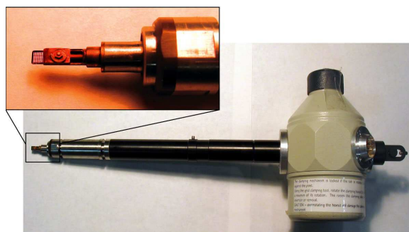
Fig. 4. View of the Gatan 630 high-tilt cryo sample holder. The dewar can be filled with liquid nitrogen to cool the sample; the specimen region is cooled by thermal conduction through a rod connecting it to this dewar. The small image shows a close-up of the tip of the holder, where a high-tilt copper grid is inserted. The grid can be retracted between two copper plates to protect cryo specimens during transfer into the vacuum chamber, and then extended so that it can be viewed at very high tilt angles (up to about \pm 80^\circ ).
