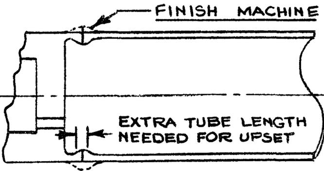
FIGURE 2 FLASH WELDED DESIGN
