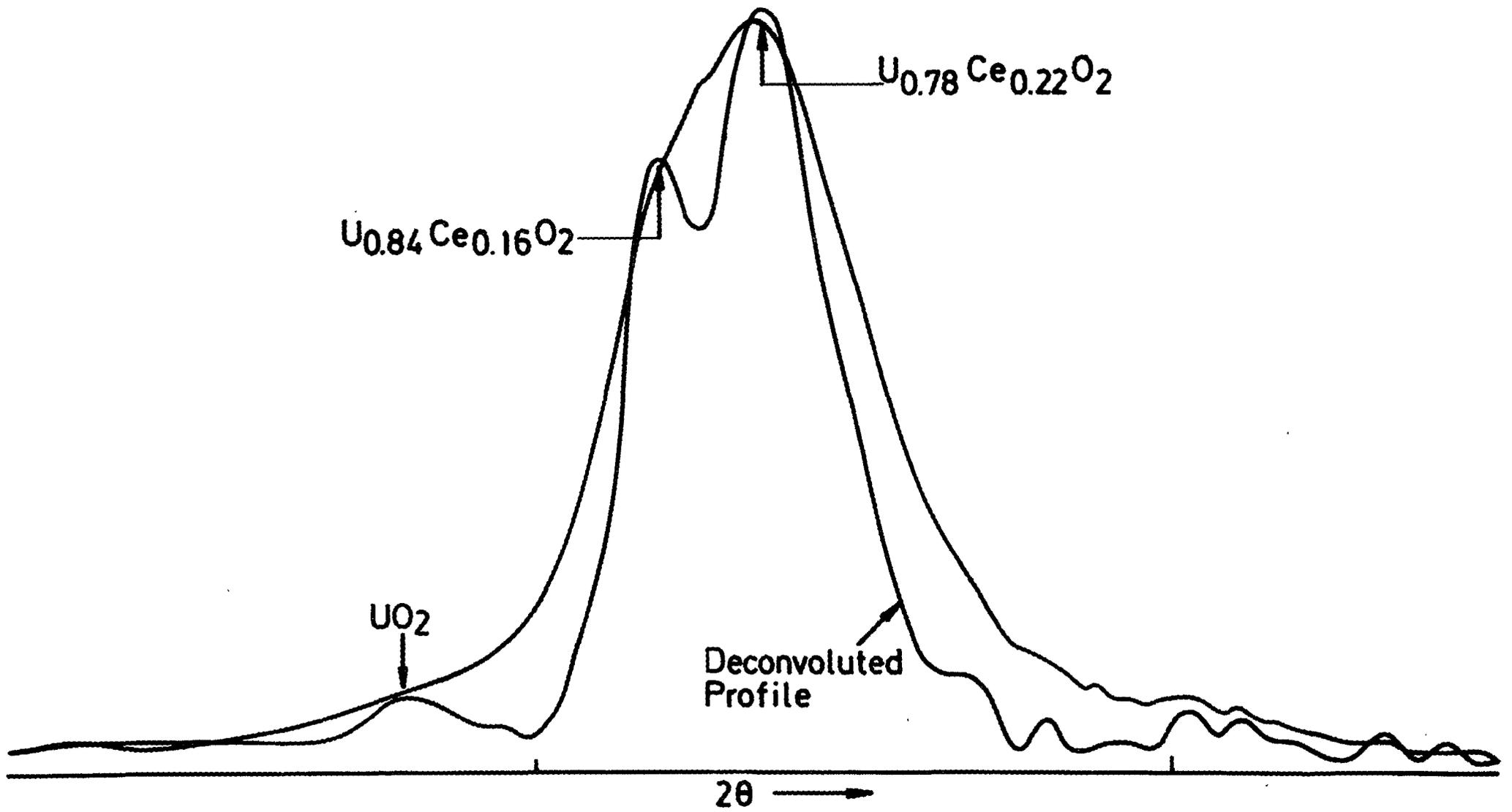
Fig.5  $K\alpha_1$  Profile of  $UO_2 - 20 CeO_2$  before and after Deconvolution
