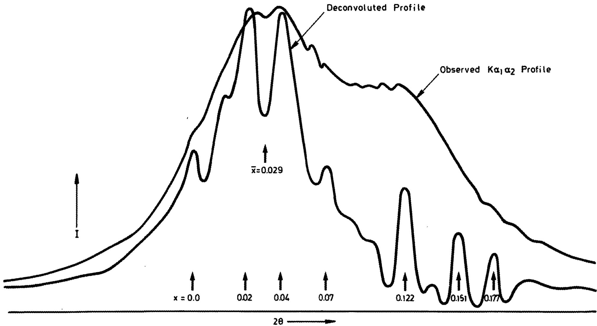
Fig.4 Observed and Deconvoluted 620 Profile of  $\text{UO}_{2+x} : \bar{x} = 0.029$
