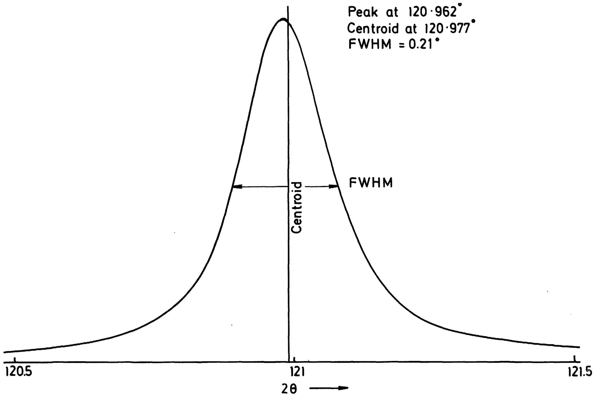
Fig.2 Diffractometer Instrument Function : ThO2 620
