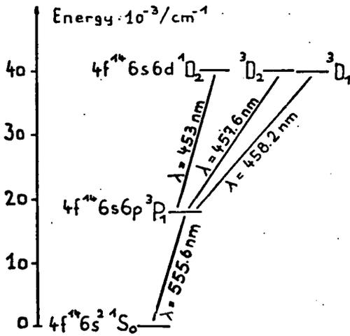
Fig.1 Part of the level scheme of the Yb-I spectrum
