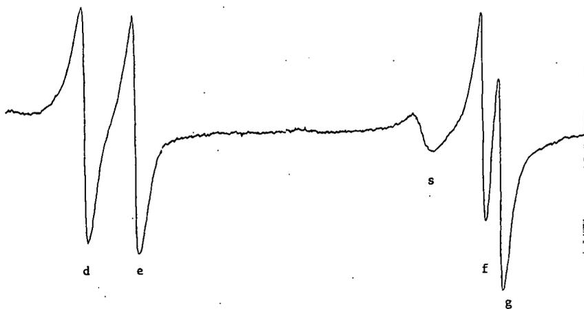
Fig. 1 : First derivative of the d, e, f, g components of the P(48)11-3 line and the s component of R(47) 9-2. The full frequency sweep is 25 MHz.
