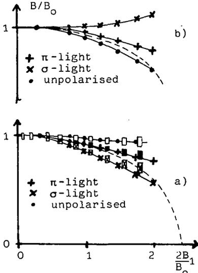
Fig.2: Position of RF resonances versus RF-amplitude (+ x • computed,  $\square$  measured, outlines indicating limits of error). a) Observation parallel to  $B_1$ . b) Observation perpendicular to  $B_1$ . The broken lines are calculated from <sup>4</sup> for the Bloch-Siegert shift of oriented atoms).
