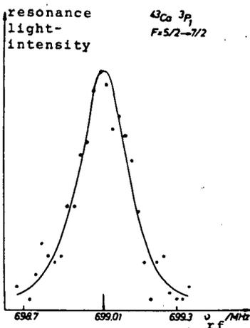
Fig.2: Radiofrequency transition  $F=5/2 \rightarrow 7/2$  in the  $4s4p^3P_1$  state in  $^{43}\text{Ca}$ .
