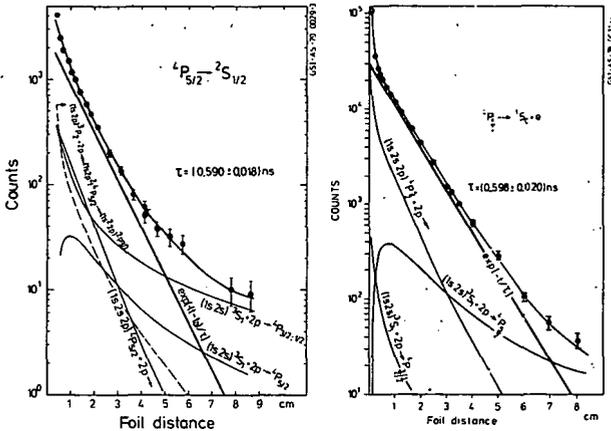
Fig. 1: Decay curves of the  $4P_{5/2}$  state observed in the x-ray (left part) and Auger electron (right part) channel. The intensity of the different contributions follows from the measured intensity of cascades.
