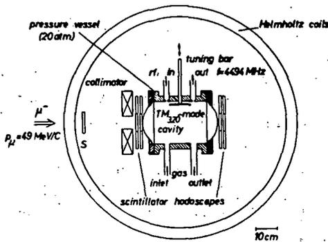
Schematic view of the  $(\alpha\mu^-e^-)$ -apparatus
