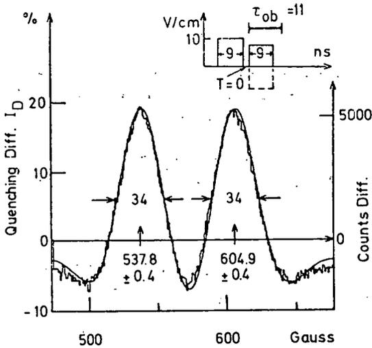
Measured difference signal of the two HFS crossings with time-separated electric fields at zero frequency, for two pulse sequences with inverted and not inverted polarity of the second pulse, without waiting-time between the pulses. The observation-time window was longer than the second pulse. The smooth line is the theoretical signal.
