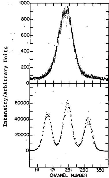
Fig. 1 : Intensity of the fluorescence light of  $^{118}\text{Cd}$  (upper part) and the  $^{114}\text{Cd}$  reference (lower part) versus the frequency of the exciting laser light.
