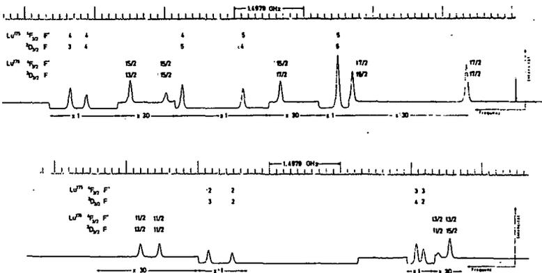
fig: Experimental curve of the hfs of the 573.7 nm line of lutetium. The frequency is increasing from right to left. The right end of the lower part continues at the left end of the upper part. For detection of the hfs components of Lu<sup>176</sup> the sensitivity of the detection circuit has been increased by a factor of 30.
