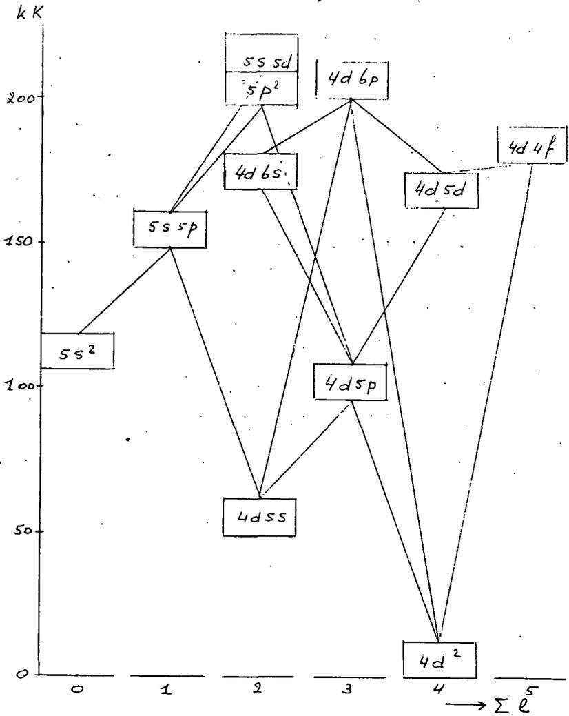
Configuration system of Nb IV and one-electron transitions.
