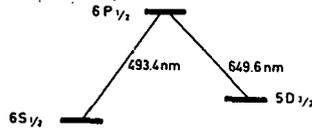
Fig. 1. Energy levels of  $Ba^+$
