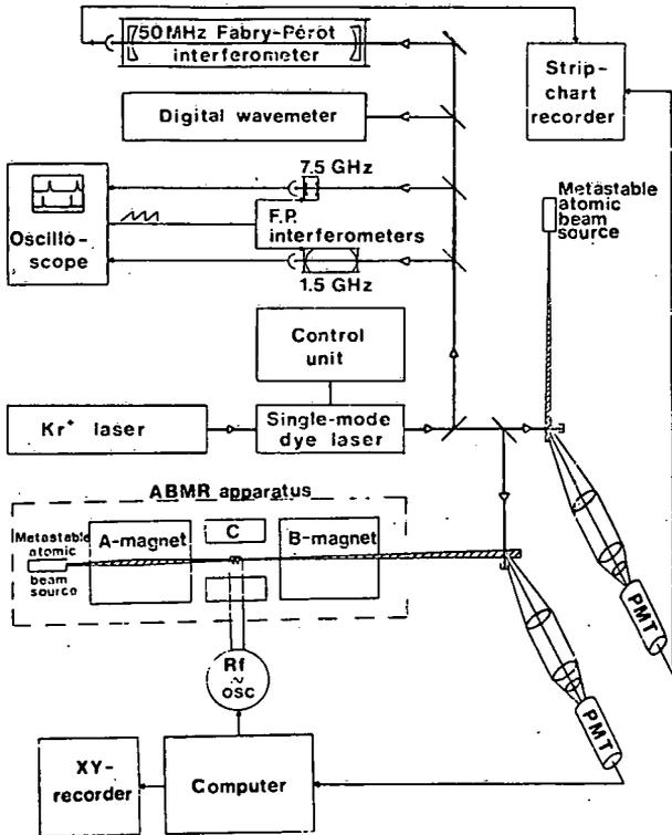
Fig. 1. Experimental set-up for fluorescence spectroscopy and atomic-beam magnetic resonance measurements.
