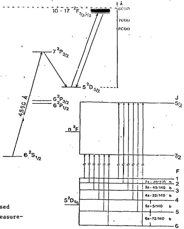
Fig. 1. Transition diagram used in high-resolution measurements on Cs atoms.
