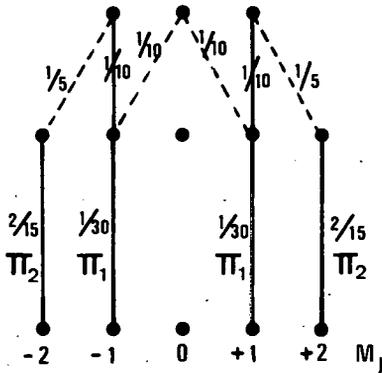
Figure 1 : Relative transition probabilities between Zeeman sub-levels in our particular three-level system. The Rabi nutation frequency is proportional to the square root of these probabilities and is thus twice as large for the  $\pi_2$  transitions as for the  $\pi_1$  transitions.
