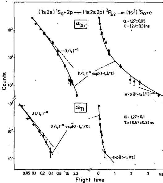
**Fig. 2:** Intensity of the  $(1s2s)^1S_0 + 2p \rightarrow (1s2s2p)^2P_{3/2} \rightarrow (1s^2)^1S_0 + e$  line. The  $(1s2s)^1S_0$  state decays by a 2E1 transition. Therefore the intensity obeys an  $\exp[-(t-t_0)/\tau] \cdot (t/t_0)^{-\alpha}$  law.
