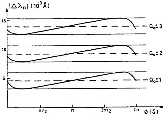
Fig. 3.- Non-sintonization effect of the finest tuning FP on the dye laser cavity modes. ( $\eta_{TW}=1.43$ ,  $d_{TW}=2.10^{-3}$  mm,  $R_{TW}=.2$ ;  $\eta_{TE}=1.36$ ,  $d_{TE}=.11$  mm,  $R_{TE}=.3$ ;  $\eta_{FTE}=1$ ,  $d_{FTE}=2$  mm,  $R_{FTE}=.8$ ;  $l=38.5$  cm, and  $\lambda=6000$  Å)
