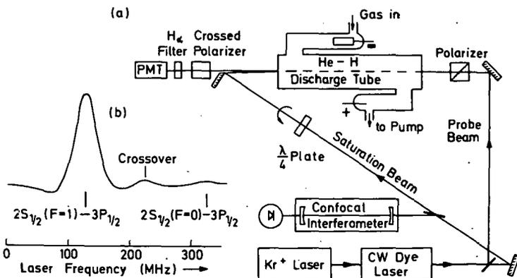
Fig. 1(a) Experimental setup for polarization spectroscopy of  $H_{\alpha}$  in a He-H dc gas discharge. (b) Polarization spectrum of the  $H_{\alpha} D_1(2S_{1/2}-3P_{1/2})$  fine structure component.
