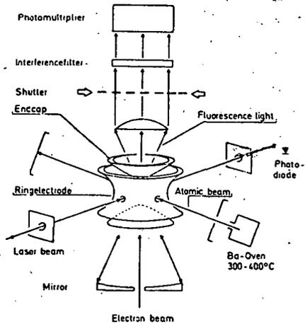
Fig. 2. Sketch of the apparatus
