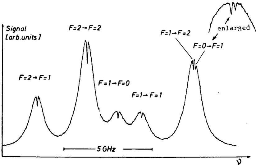
Resonance fluorescence and Lamb dip signals of the  $2^3S_1-2^3P_1$  transition in  ${}^6\text{Li}^+$ .
