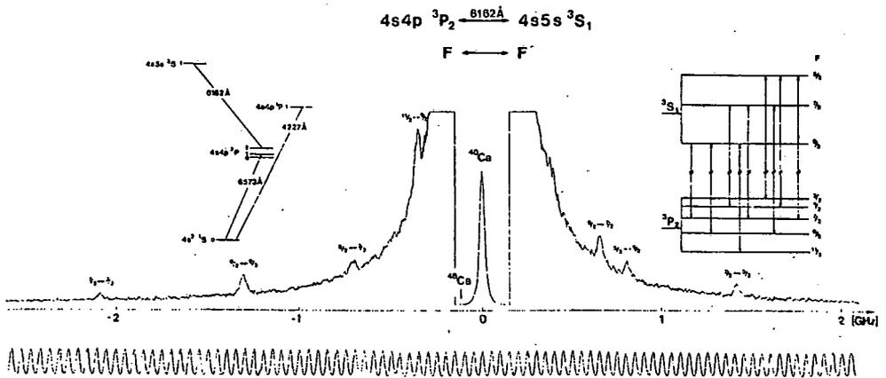
Fig. 2. High-resolution laser scan of the 6162 Å Ca line, displaying the hyperfine structure for  $^{43}\text{Ca}$ .
