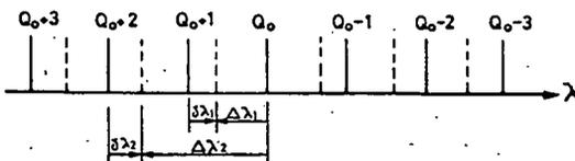
Fig. 1.- Scheme of resonator modes and their shift by effect of internal tuning elements.
