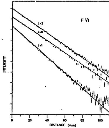
Fig. 1. Intensity decay curves for the  $2s3p\ ^3P_{0,1,2}$  levels in F VI. All curves were taken with the same initial statistics, about 10 000 counts/channel at the position closest to the foil, but are shifted for purposes of illustration. The ordinate scale is logarithmic.
