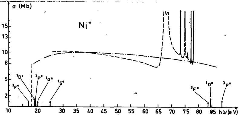
Figure 2:  $\sigma_{3d}$  of  $Ni^+$  ----- our R matrix(D.L.) calculations
