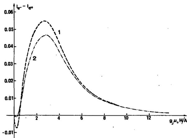
Fig. 1. Intensity difference of the circularly polarized components of the resonance fluorescence excited with  $\pi$  polarized  $D_2$  line, with  $I_{\pi} + I_{\sigma^-} + I_{\sigma^+} = 1$ ,  $B \approx 0$ :
