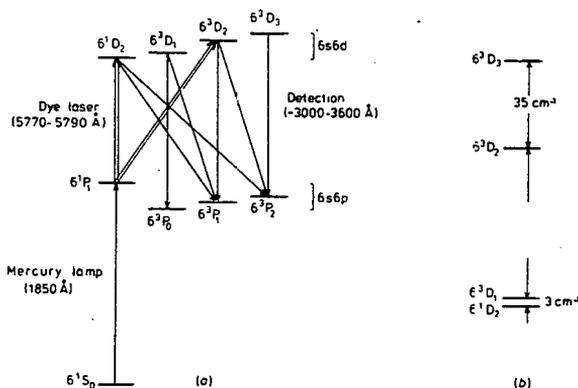
Figure 1. Mercury levels involved in the experiment: (a) simplified Grotrian diagram showing excitation and detection lines. (b) relative positions of  $6s6d$  levels (to scale).
