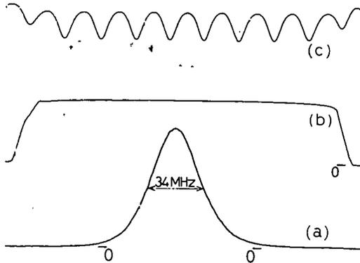
Fig. 1 - Trace (a) : Typical experimental recording of the probe signal (temperature : 77 K ; Kr pressure : 17 mT). Trace (b) : Output level of the frequency-scanning Xe laser. Trace (c) : Reference fringes, separated by 20.85 MHz.
