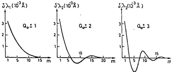
Fig. 2.- Shift of the three first modes as a function of the duration of a short rectangular pulse ( $\eta=1$ ,  $d=4.35$  mm,  $R=.8$ , resonator length  $l=10$  cm, and  $\lambda=6000$  Å).
