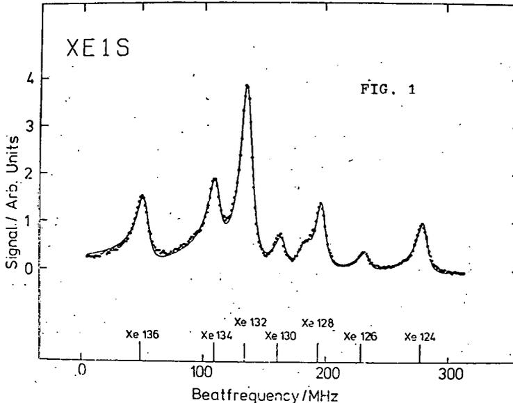
Fig. 1 shows a typical spectrum of all even stable xenon isotopes obtained after two frequency scans. The solid line represents a least-squares fit to the experimental data represented by the dots in Fig. 1.
