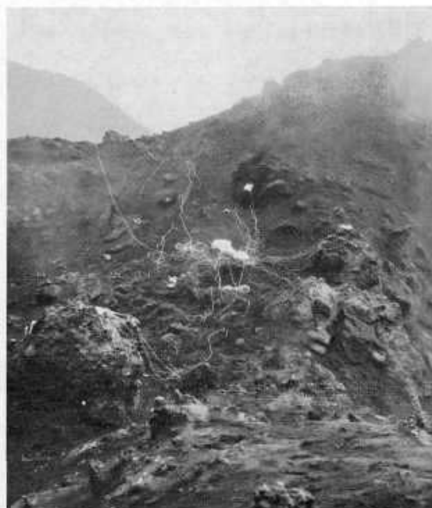
Fig. 5. Northernmost part of "Surtur I" with temperature recording instrument (cf. fig. 2: 1-9). To the left, probes 18a, 19b, 20a and 21b (fig. 2: 8, 9). To the right, rim of crater, position of probes 7a and 8b (fig. 2:4). Behind the instrument, which was protected by a plastic envelope, are probes 1a, 2b, 9a, 10a and 11b (fig. 2:1, 5). — 15. 8. 1972, E. Sjn.
