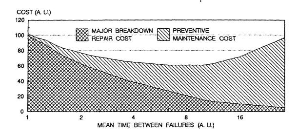
Fig. 9.1 Typical measuring instrument maintenance cost distribution versus mean time between failures.
