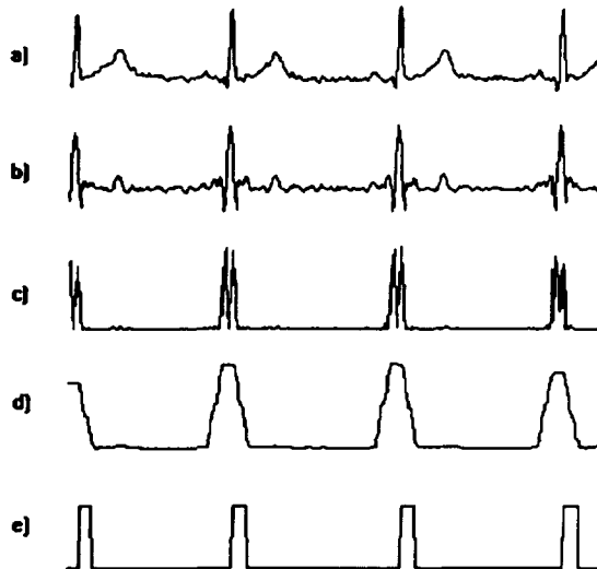
FIG.6. QRS width algorithm determination. a) Original ECG signal. b) SQ. c) Output of differentiation and squaring. d) Moving-window integration output. e) QRS width output pulse.
