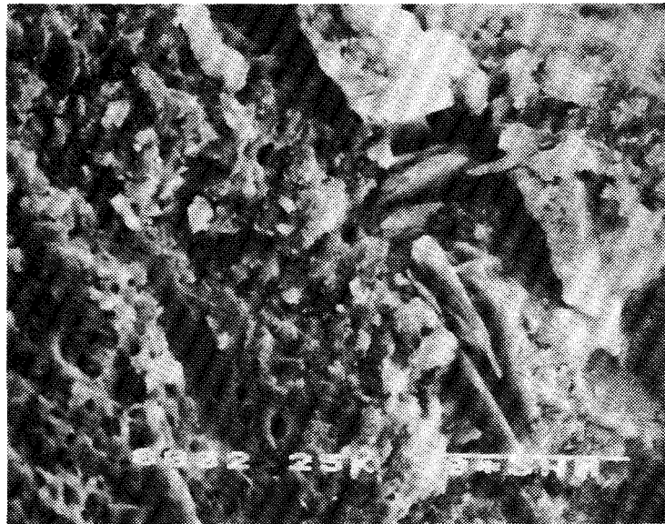
Figure 51. Scanning electron photomicrograph (SEI) of the interface between lightweight aggregate and cement paste when cement paste type 2 was used. Concrete sample: 222 (1 min). The area to the left is aggregate and the area to right is cement paste. Original magnification: x 1000, the picture width: 100 \mu m.
