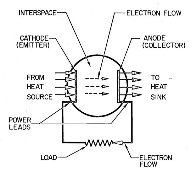
Figure 1. The Essentials of a Thermionic Energy Converter
