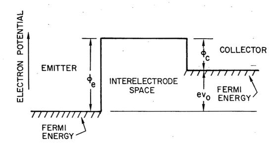
Figure 2. Potential Energy Diagram for an Idealized Converter
