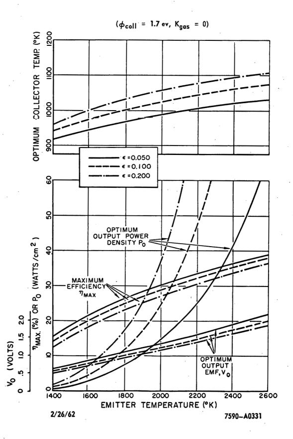
Figure 3. Performance Parameters for an Idealized Converter
