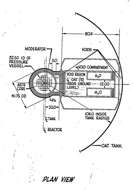
Figure I. Internal Geometry of the OAT
