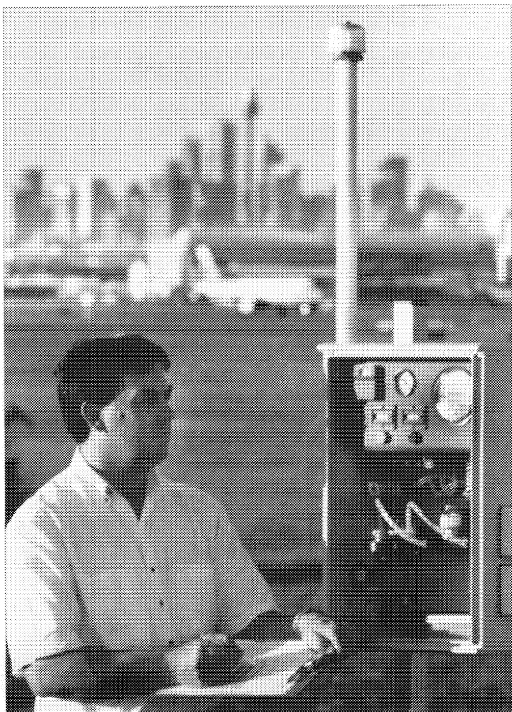
David Garton checking an ANSTO aerosol sampling monitor at Sydney's Kingsford Smith Airport, one of a chain of monitors in major urban areas of New South Wales.
