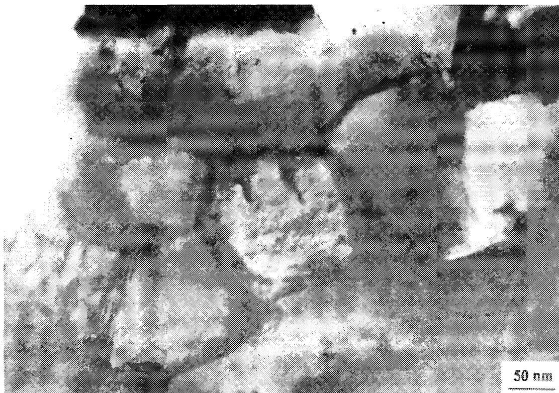
Figure 3 Transmission Electron Micrograph of the rim of a high burn up LWR fuel sample, showing the restructuring into a fine scale subgrain structure, free of dislocations or fission product precipitation
