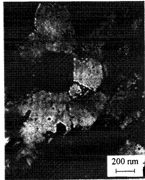
Figure 4: TEM micrograph of FeAl40 Grade 3
