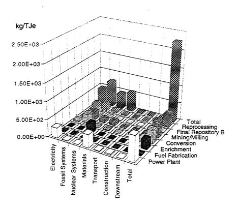
Fig. 4. CO<sub>2</sub> emissions from nuclear FENCH in UCPTE.
