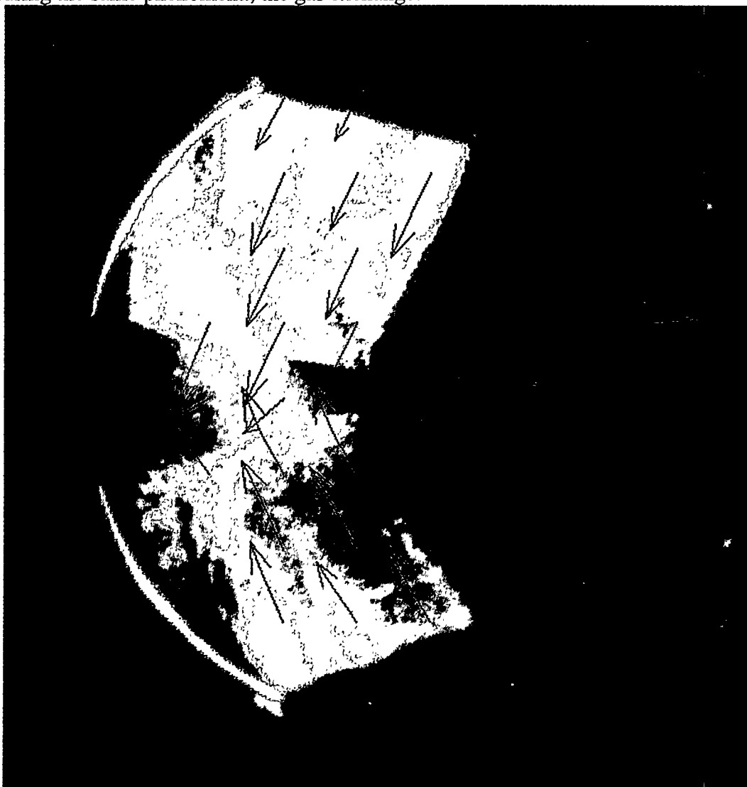
Figure 38. Arrows visualising the flow velocities from the transfer ports(measured with LDV) placed in the same figure as a Laser Sheet Droplet Illumination image. This image was captured as the piston position was at BDC. The cylinder was the J630 cylinder (cup handle transfer channels) [12,13].
