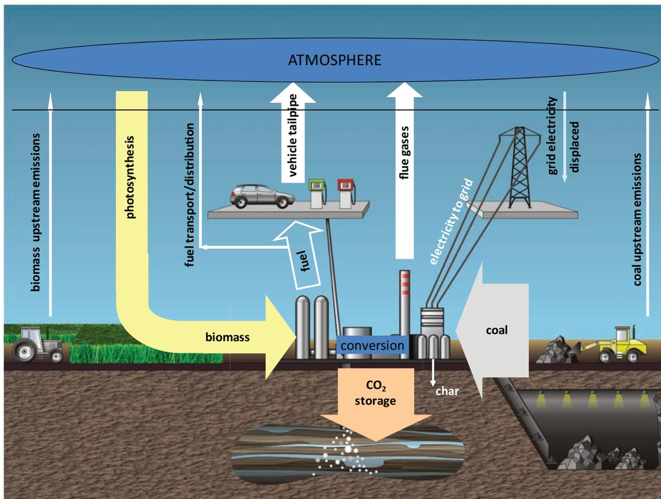
**Figure SPM-8.** | Carbon flows for conversion of coal and biomass to liquid fuels and electricity. For this system, when biomass is approximately 30% of the feedstock input (on a higher heating value basis), the net fuel cycle GHG emissions associated with the produced liquid fuels and electricity would be less than 10% of the emissions for the displaced fossil energy. Source: Larson et al., 2010, see Chapter 12.<sup>5</sup>
