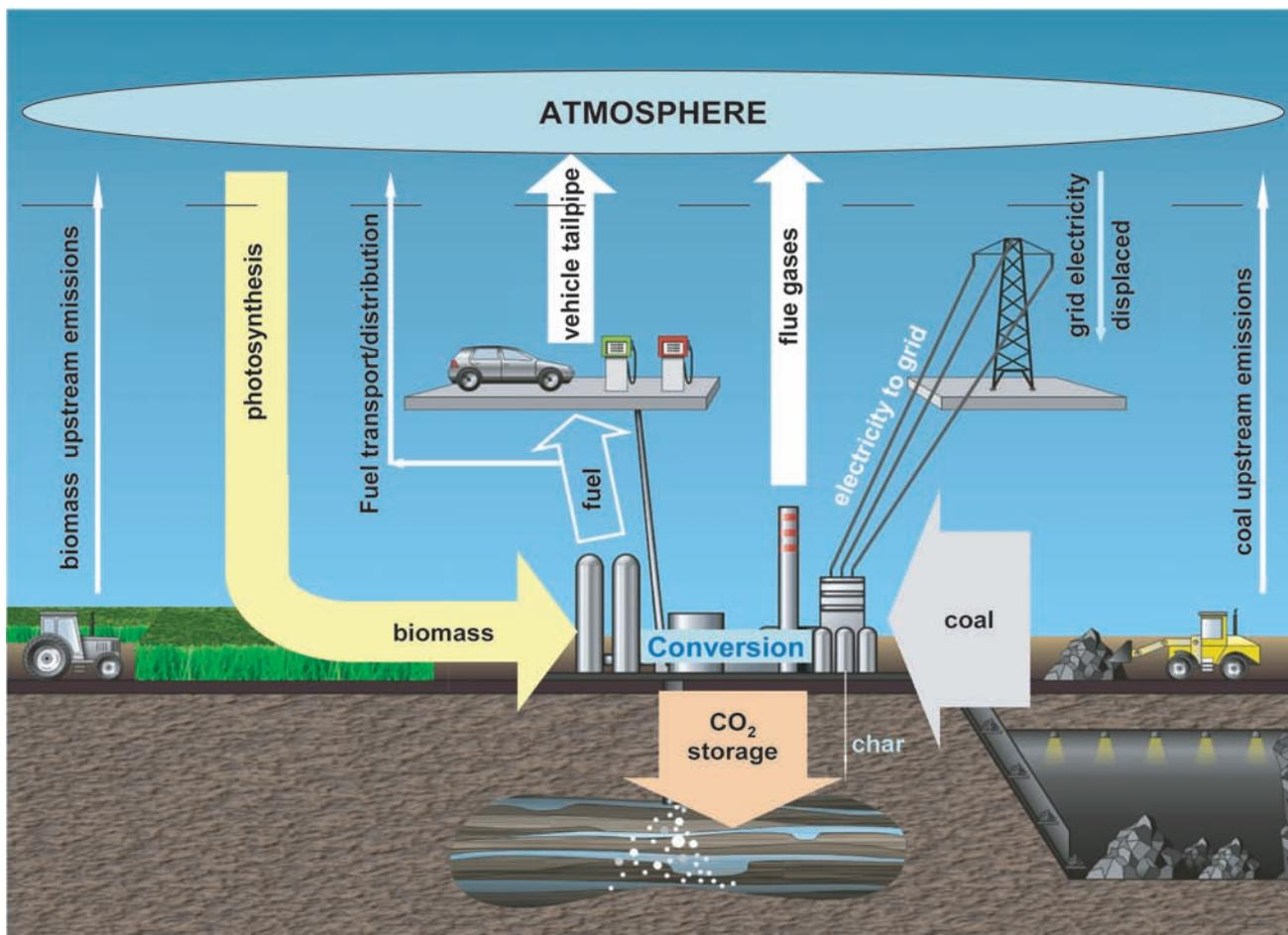
**Figure TS-20** | Carbon flows for conversion of coal and biomass to liquid fuels and electricity. When biomass is approximately 30% of the feedstock input (on a higher heating value basis), the net fuel cycle GHG emissions associated with the produced liquid fuels and electricity would be less than 10% of the emissions for the displaced fossil energy. Source: Chapter 12.<sup>24</sup>
