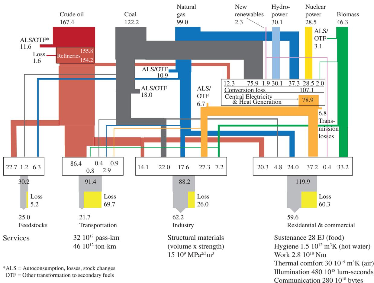
**Figure TS-10 |** Global energy flows (in EJ) from primary to useful energy by primary resource input, energy carrier (fuels), and end-use sector applications in 2005. Source: data from IEA, 2007a; 2007b (corrected for GEA primary energy accounting standard) and Cullen and Allwood, 2010, see Chapter 1.<sup>13</sup>
