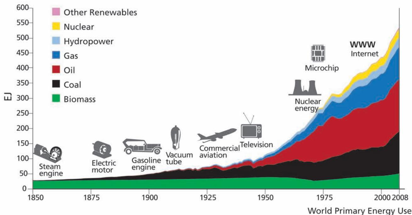
**Figure SPM-1.** | Evolution of primary energy shown as absolute contributions by different energy sources (EJ). Biomass refers to traditional biomass until the most recent decades, when modern biomass became more prevalent and now accounts for one-quarter of biomass energy. New renewables are discernible in the last few decades. Source: updated from Nakicenovic et al., 1998 and Grubler, 2008, see Chapter 1.<sup>1</sup>
