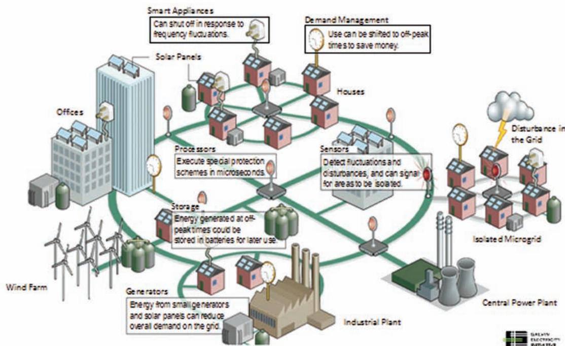
**Figure TS-22** | Example of a smart grid, a network of integrated microgrids that can monitor and heal itself. Source: Amin, 2008; see Chapter 15.<sup>30</sup>
