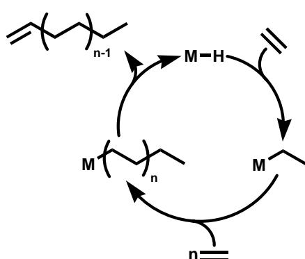
In case of the  $\alpha$ -SABLIN technology, the ratio of catalyst and cocatalyst is strongly affecting this distribution and can be easily controlled in order to tune the desired product distribution. This features allows an enormous flexibility of the process to react to changing market demands for lighter or heavier LAO fractions.
