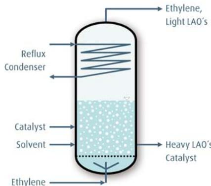
Ethylene is introduced via a gas distribution system to the bottom section, whereas the liquid heavy LAO, together with the solvent and the catalyst, are withdrawn from the bottoms. The LAO reaction is highly exothermic. By removing this heat with the ethylene, heat exchanger surfaces within the reaction area, which would be subject to heavy fouling, are avoided. The function of ethylene as a coolant in the LAO reactor is a unique feature of the  $\alpha$ -SABLIN technology.
