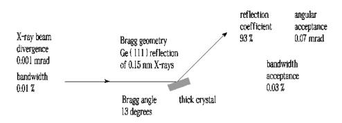
Fig. 4. Concept of the photon beam deflector for the LCLS X-ray transport system based on the use of a crystal in Bragg reflection geometry.
