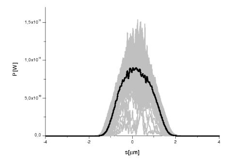
Fig. 21. Power distribution of the X-ray radiation pulse in the case of undulator tapering. Here the output undulator is 21 - cells long and composed of 9 uniform and 12 tapered cells. Grey lines refer to single shot realizations, the black line refers to the average over a hundred realizations.
