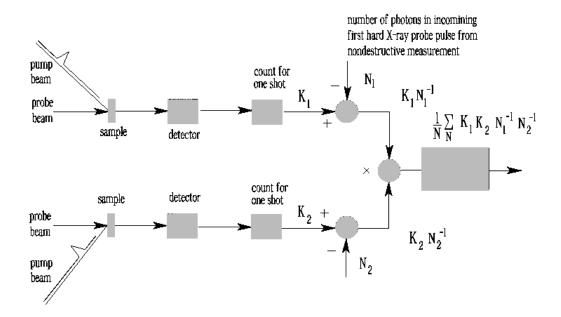
Fig. 31. Correlation apparatus for analysis of sample dynamics.
