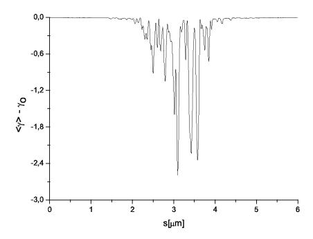
Fig. 9. Electron beam energy loss after the SASE undulator (11 cells). The data refers to a single typical realization.
