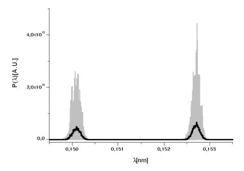
Fig. 34. Pump-probe experimental setup. Spectrum of double hard X-ray probe pulse. Here the first undulator is11- cells long and resonant at 0.1500 nm wavelength. The second undulator is 12- cells long and resonant at 0.1527 nm wavelength. Grey lines refer to single shot realizations, the black line refers to the average over a hundred realizations. The two colors are clearly visible.
