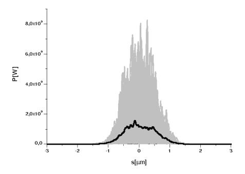
Fig. 33. Pump-prob experimental setup. Power distribution of the second X-ray radiation pulse. Here the second undulator is12 - cells long and resonant at 0.1527 nm wavelength. Grey lines refer to single shot realizations, the black line refers to the average over a hundred realizations.
