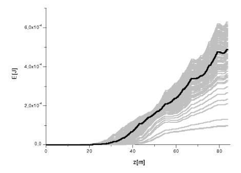
Fig. 19. Energy in the X-ray radiation pulse versus the length of the output undulator in the case of undulator tapering, Here output undulator is 21 - cells long, and composed of 9 uniform plus 12 tapered cells. Grey lines refer to single shot realizations, the black line refers to the average over a hundred realizations.
