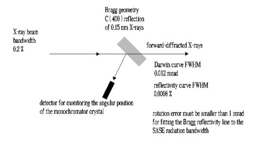
Fig. 3. Alignment of the wake monochromator crystal.
