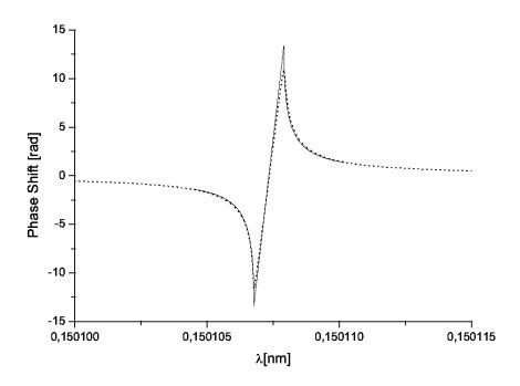
Fig. 8. Phase relevant to the Bragg (400) diffraction of X-rays at 0.15 nm from a Diamond crystal with a thickness of 0.1 mm,  $\sigma$ -polarization component. The phase retrieved according to the minimal phase method (dotted line) is compared with the phase obtainable with the help of Eq. (14)
