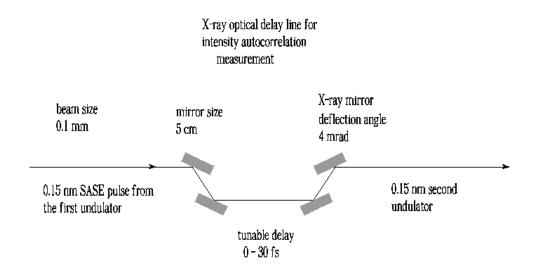
Fig. 25. X-ray optical system for delaying the SASE X-ray pulse with respect to the electron bunch. The X-ray optical system can be installed within the magnetic chicane of the self-seeding setup in placed of the single crystal monochromator.
