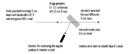
Fig. 5. Bragg transmission X-ray phase retarder based on a 0.2 mm thick diamond crystal at 8 keV. The Diamond (111) reflection is used. A linearly polarized, monochromatic X-ray beam is directly converted to circularly-polarized X-ray beam.
