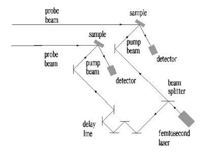
Fig. 29. Sketch of principle for the optical pump/hard X-ray probe technique based on the use of time jitter between double pump and double probe pulses. This technique exploits two spatially separated samples and records the correlation of the counts for each value of the delay between two pump-laser pulses.
