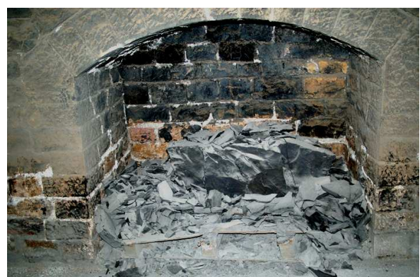
Figure 3.56: Disintegrating rock sample. This rock with an extent of approximately 1.5 m is located uncovered since over ten years in a niche of the old tunnel.
