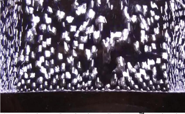
Figure 6: Steady-state Film and Nucleate Boiling in Novec™ 649. The ends of the wire have quenched, whereas the center remains in the film boiling regime.
