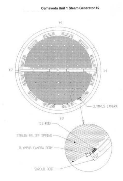
Figure 4: Camera location was confirmed close to X-1 port.
