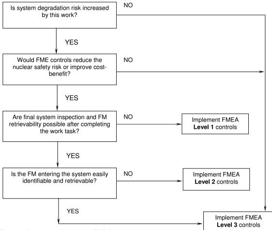
Figure 1: Determining Appropriate FME Control Levels
