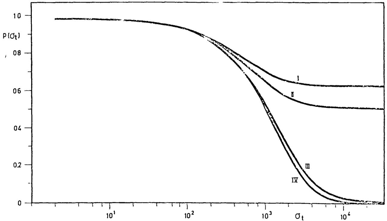
Figure 1: Penetration Probability as Function of Absorber Cross Section
