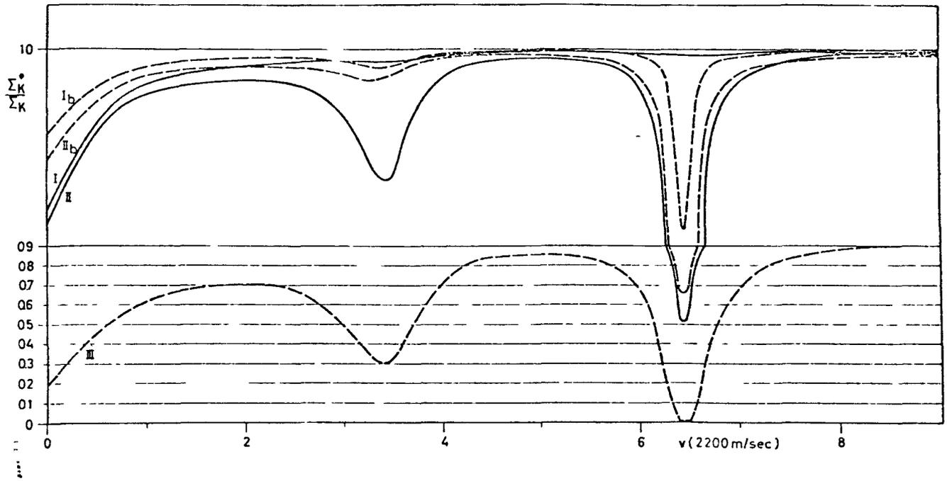
Figure 3: Ratio of the Effective Kernel Material Total Cross Section  $\Sigma_K^*$  to the  $\Sigma_K$  of Homogenized Medium.
