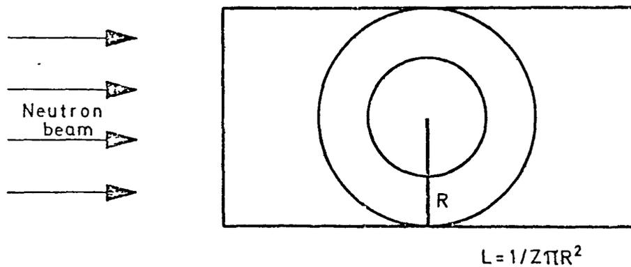
Figure 2: Model for a Neutron Beam through the Area of one Coated Particle
