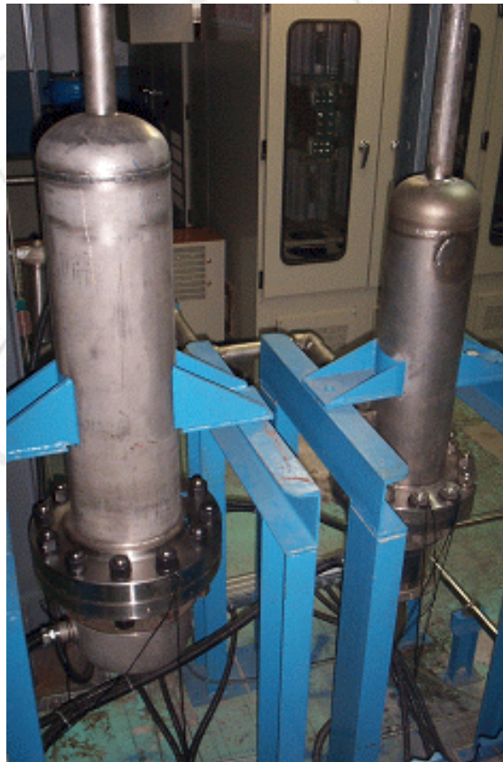
Figure 2-4. Photograph of pre-heater
