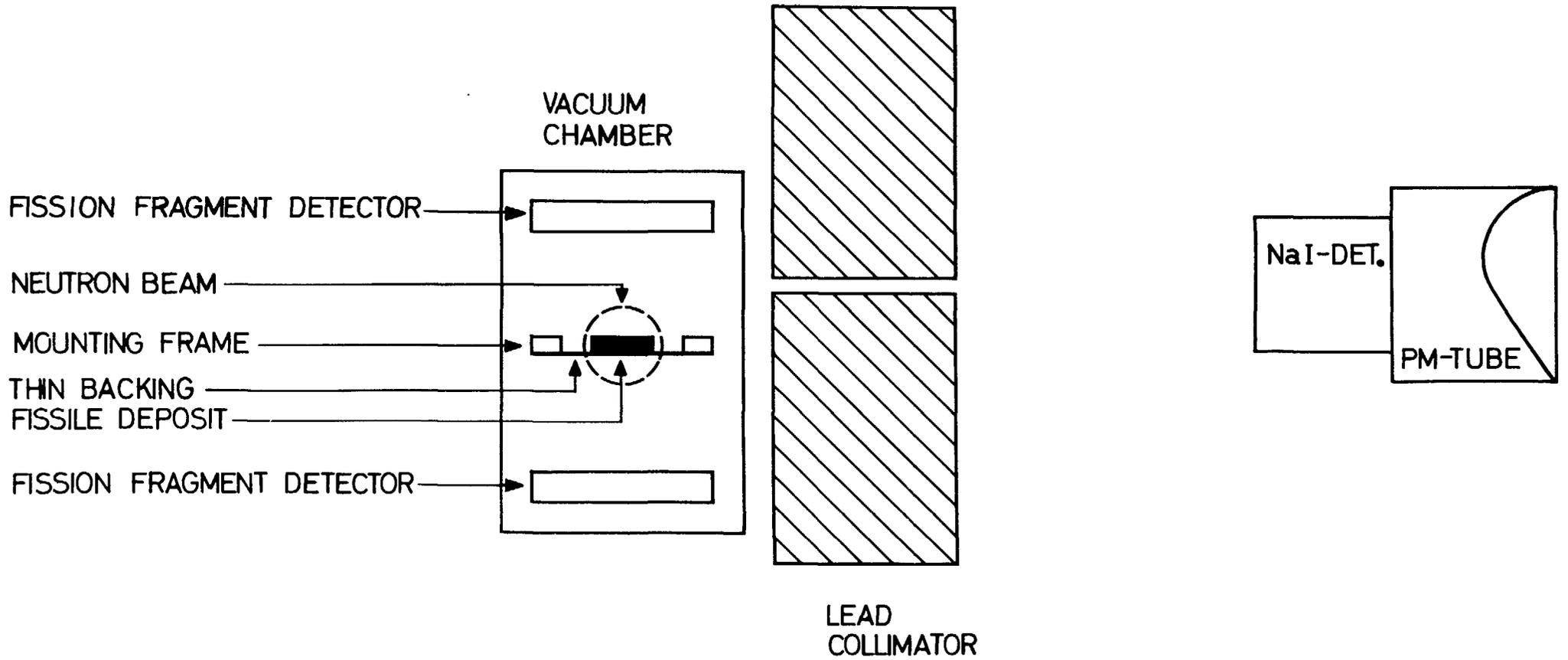
Fig. 1. Schematic diagram of the experimental arrangement
