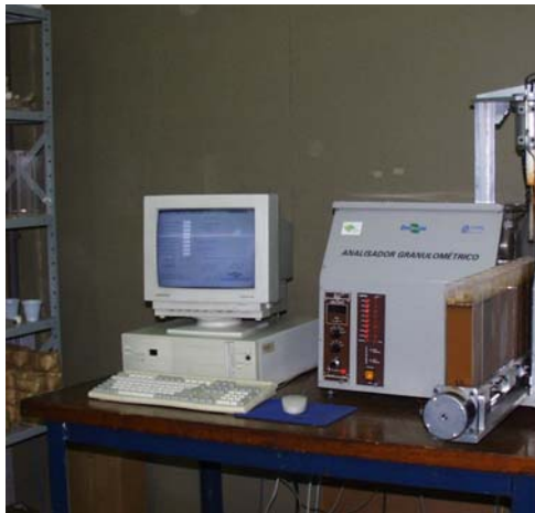
Figure 1. Equipment for multiple soil physical parameters determination.
