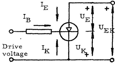
Fig. 2.1. The common collector transistor switch.
