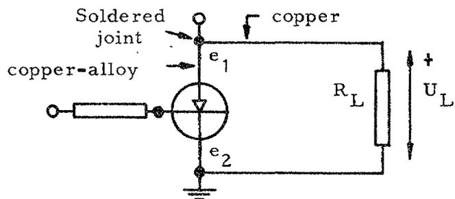
Fig. 7.1. Thermoelectric voltages in the switch.
