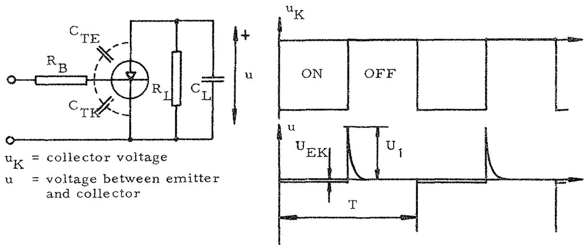
Fig. 5.1. Spikes appear over the switch at switching on and off.
