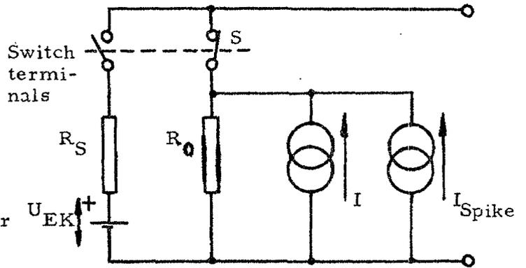
Fig. 2.2. The equivalent circuit of the low level switch.
