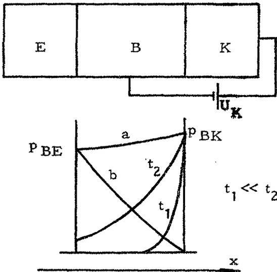
Fig. 2.3. The excess hole density distribution in the base with open emitter after a positive voltage  $U_K$  has been impressed between the collector and the base.
