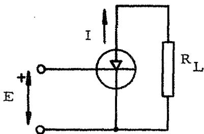
Fig. 4.1. The switch in the off state with large reverse voltage.
