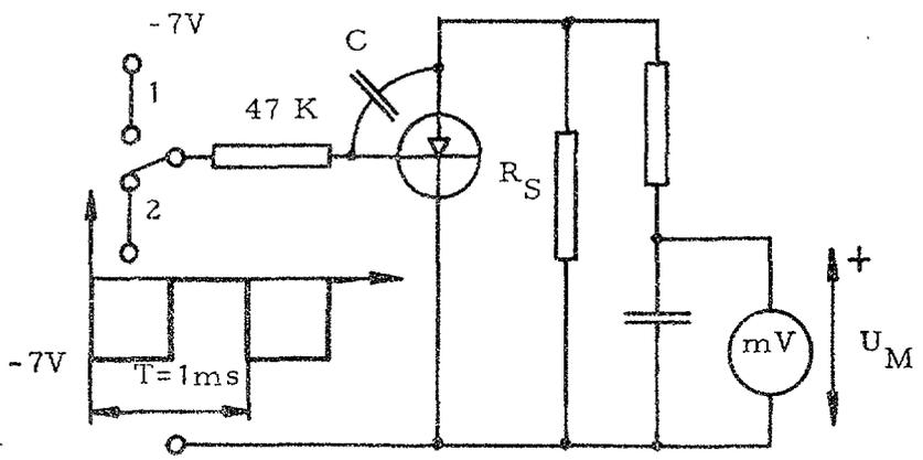
Fig. 5.3. Circuit for the measurement of  $U_{SPOFF}$
