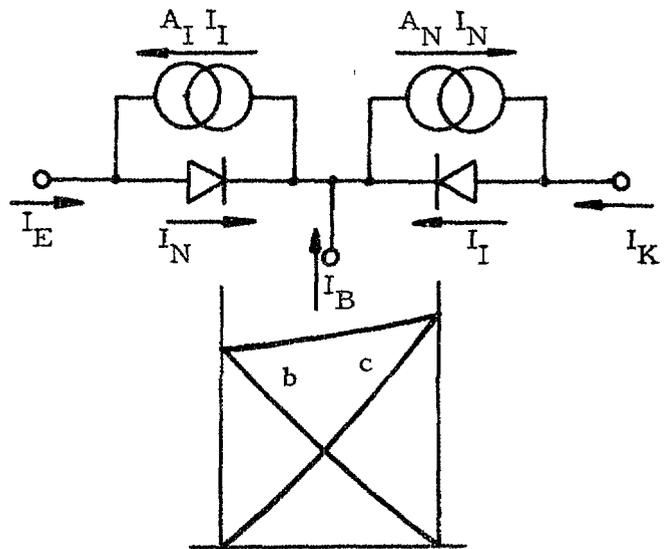
Fig. 2.4. The double diode equivalent circuit. This is derived by superposing two excess hole density distributions shown by curves b and c.
