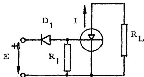
Fig. 4.2. The switch in the off state with small reverse voltage.
