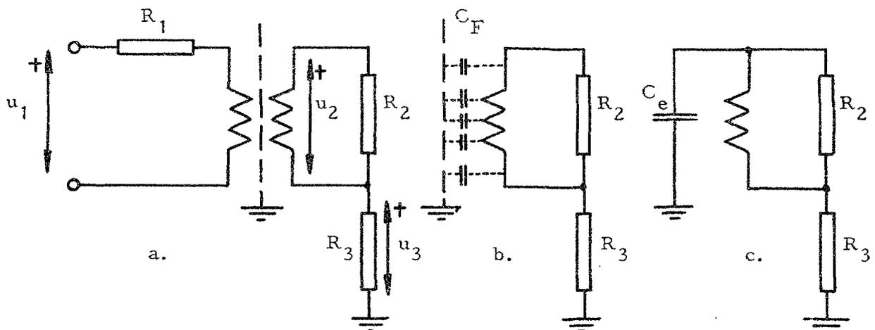
Fig. 6.1. a. Drive circuit with a transformer.
